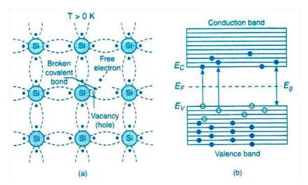
Figure 5.3 Silicon crystal at temperature above 0K (a) Due to thermal energy breaking of Covalent bonds take place (b) Energy band representation
