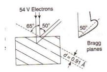
Fig. 4.1(c) Bragg planes in Nickel crystal
