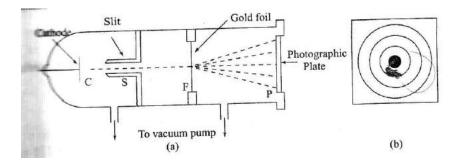
Fig 4.2: (a) G.P.Thomson's Apparatus, (b) pattern recorded on the photographic plate
