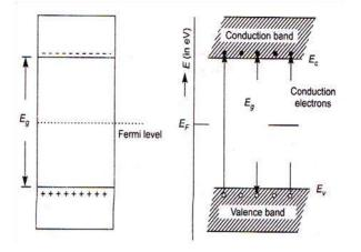
Figure 5.1 (a) Energy band diagram of a semiconductor (b) Fermi level at T=0K & Thermal excitation of electrons at T>0K
