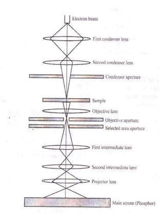
Fig. 3.7 Schematic representation of TEM.
