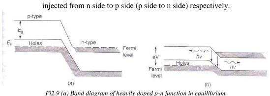
(a) Band diagram of heavily doped p-n junction in equilibrium) (b) Band diagram of heavily doped p-n junction with forward bias
