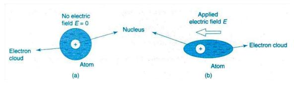
*Fig. 1.8 (a) Un polarized atom in the absence of field (b)Electronic polarization due to distortion of electron cloud by the field E*
