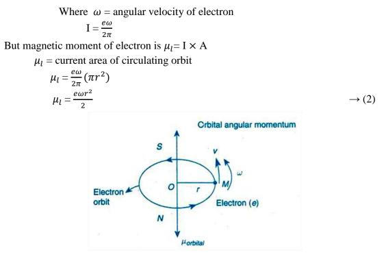
Fig. 1.13 Orbital magnetic moment of electrons
