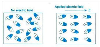
Fig. 1.6 Polar dielectric orientation without field and with field.
