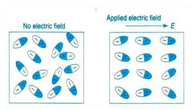
Fig. 1.10: Orientational polarization
