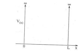
Fig.4.4 Square potential well infinite height
