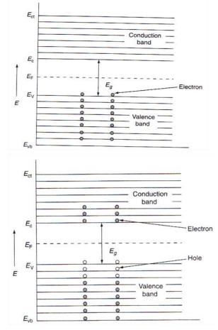
Figure 5.5 (a) Energy band diagram of silicon at T = 0K(b) Energy band diagram of silicon at T > 0K
