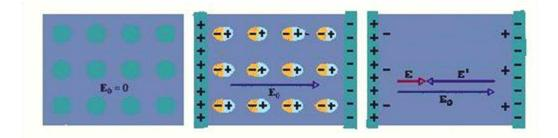
Fig. 1.5 (a) non polar dielectric in E=0 (b) Non polar dielectric when 'E' is applied (c) Totally polarized non polar dielectric with net field
