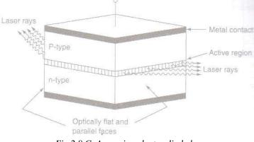
Fig.2.8 GaAs semiconductor diode laser
