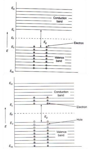
Figure 5.4 (a) Energy band diagram of silicon at T = 0K(b) Energy band diagram of silicon at T > 0K
