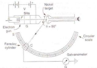
Fig 4.1(a) Davisson and Germer's experimental arrangement for verification of matter waves
