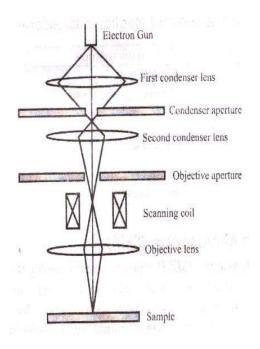
Fig.3.6 Schematic representation of SEM
