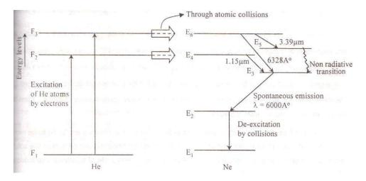
Fig.2.4. Energy level diagram of He-Ne atoms.
