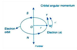
Fig.1.12 Revolving electron in an atom produces magnetic moment
