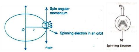
Fig. 1.14 Spin magnetic moment of electrons
