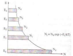
Fig.2.2 Boltzmann distribution for several energy levels
