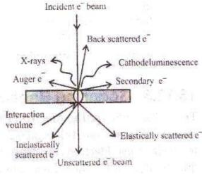
Fig.3,5 Specimen interactions in SEM
