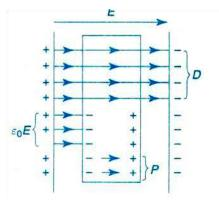
Fig. 1.4 Electric lines of forces in a polar dielectric
