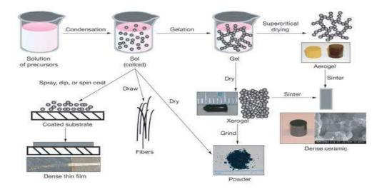
Fig. 3.1 Schematic of Sol-Gel method
