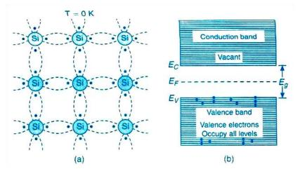
Figure 5.2: Intrinsic silicon crystal at T = 0K(a) 2-D representation of silicon crystal (c) Energy band diagram of intrinsic semiconductor
