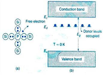
Figure 5.7 (a) Representation of n-type silicon at T = 0K (b) Energy band diagram at T = 0K
